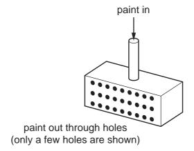
The paint is ejected at a speed of 2.5 m s<sup>-1</sup> through 400 holes, each of area 0.4 mm<sup>2</sup>. The density of the paint is  $900 \,\mathrm{kg}\,\mathrm{m}^{-3}$ .
