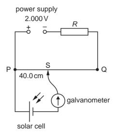
The potentiometer wire PQ is  $100.0 \, \text{cm}$  long and has a resistance of  $5.00 \, \Omega$ . The power supply has an e.m.f. of  $2.000 \, \text{V}$  and the solar cell has an e.m.f. of  $5.00 \, \text{mV}$ .
