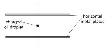
As some of the oil evaporates, the droplet loses mass and starts to accelerate. Its charge remains constant.
